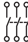
No Fuse, Two-pole, 240 Volts AC; 250 Volts DC (100-600 amps only); Three-pole, 240 Volts AC or Two-pole with Switching Neutral
